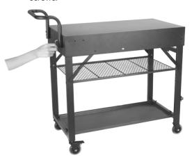
4. Install the handle on the left side of the grill cart (near the bottle opener) and secure it with the screws.
